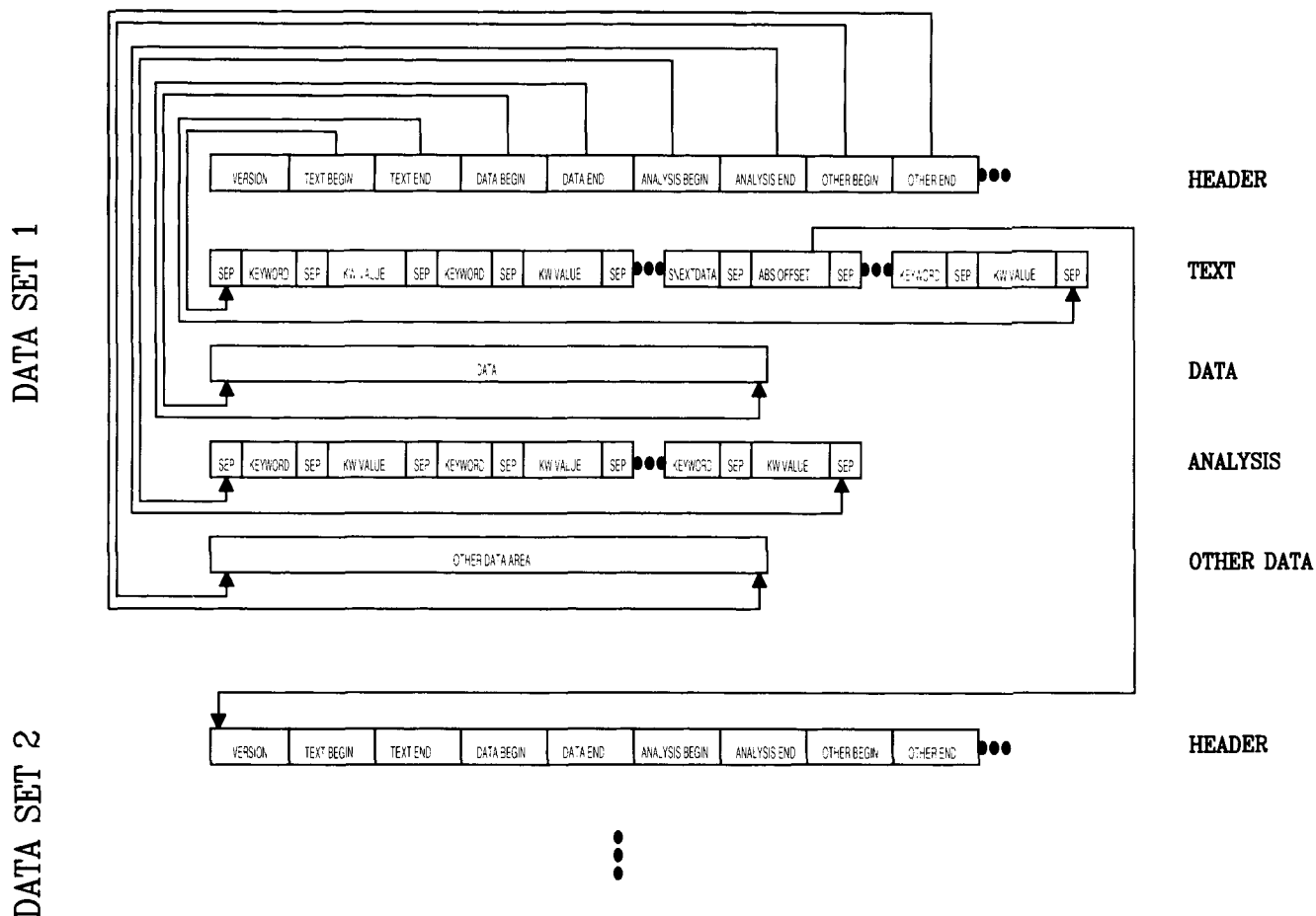
FIG. 1. The structure of an FCS 2.0 Standard Data File. All parts of the file are included, with arrows indicating the way the byte offsets point to the beginning and end of each part. In the HEADER part, the OTHER BEGIN and OTHER END offsets show how the user can
